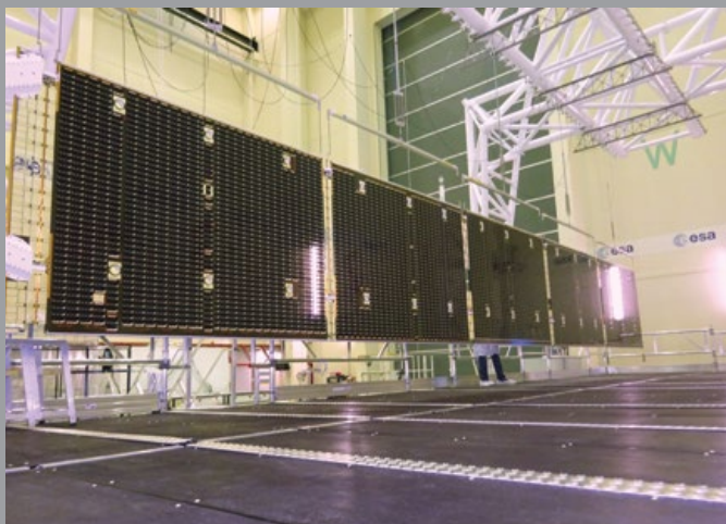
BepiColombo Mercury Transfer Module solar array wing in the zero-g rig during preparation for integration
