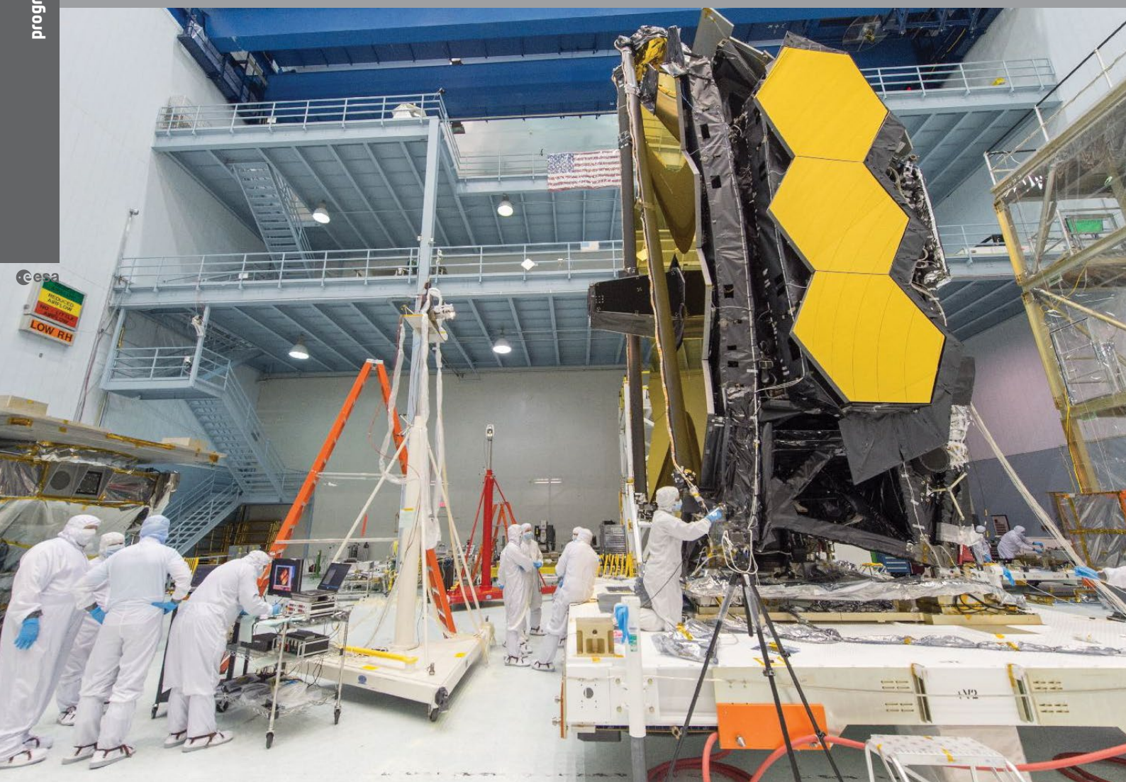
Inspection of the JWST NIRSpec micro-shutter array through the telescope optics. The telescope wings are folded in launch configuration (NASA)
